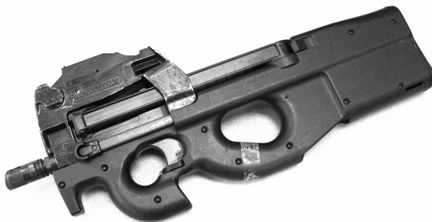
Figure 4.25 The Fabrique Nationale P-90 submachine gun chambered in the FN 5.7×28mm. The P-90 is a classic bull-pup design. The PS-90 is a commercially available semiautomatic copy. The PS-90 is fitted with a 16.1-inch barrel, although conversion to the short submachine gun barrel is not difficult. (Image from author's collection.)
